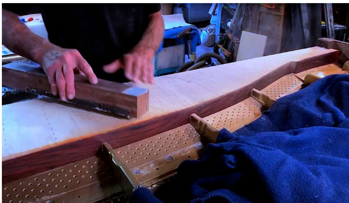
Illus.10 The pinblock being refinished
