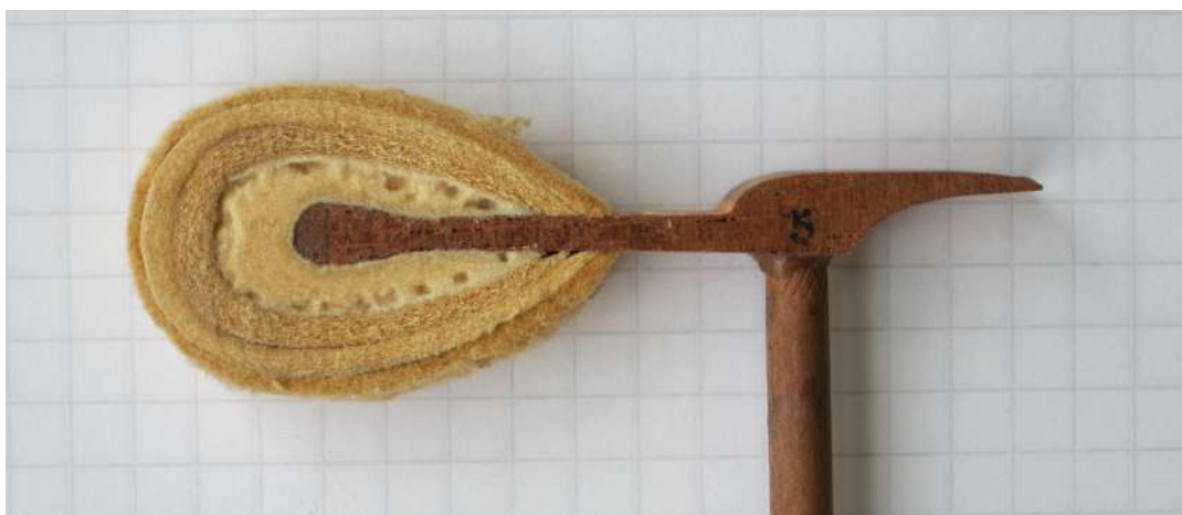
Illus. 15 Pleyel grand piano: detail of an original hammer with felt underlay and chamois leather top layer
