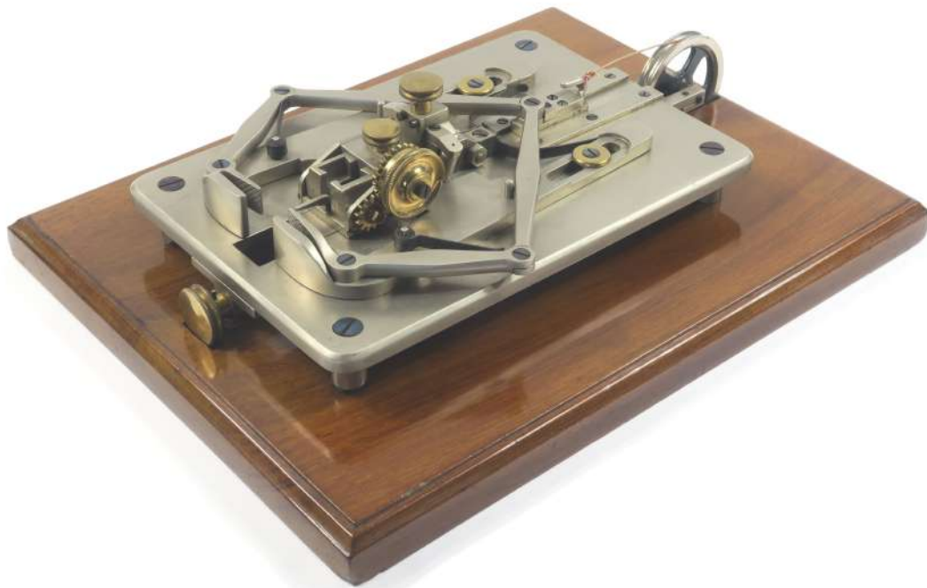
Illus.6 Model of a hammer covering machine, Pinet factory, Paris (end of the 19th century), Musée de la Musique, E.977.1.2
