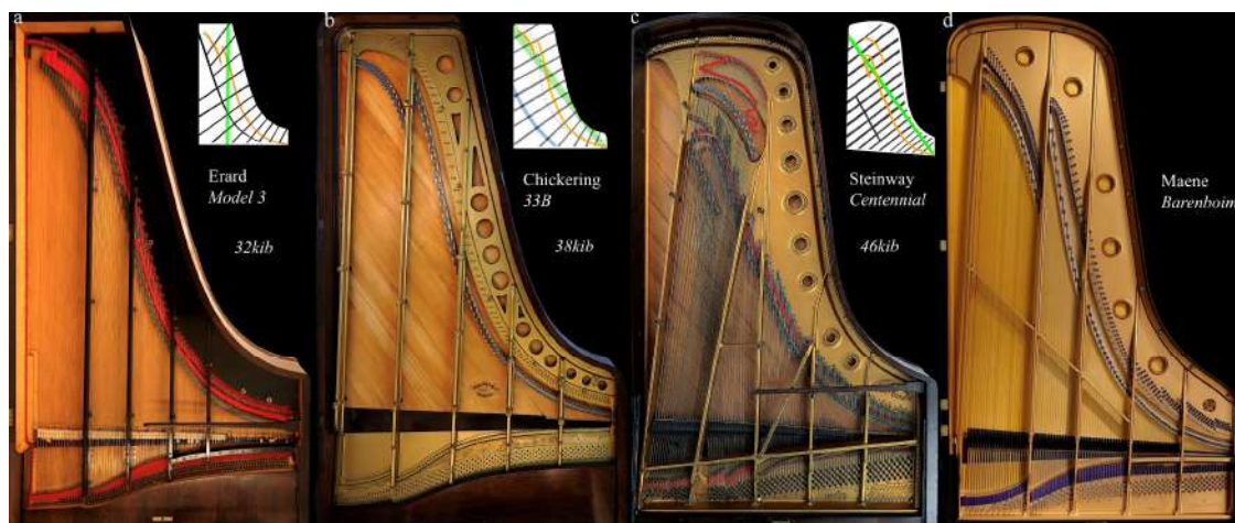
Illus.7a-d Grand pianos by Erard, Chickering, Steinway and Maene, soundboard view. In the schematic inserts, black indicates ribs, green is the wood grain orientation of the board, blue is the bass cutoff bar, and brown is the bridges
