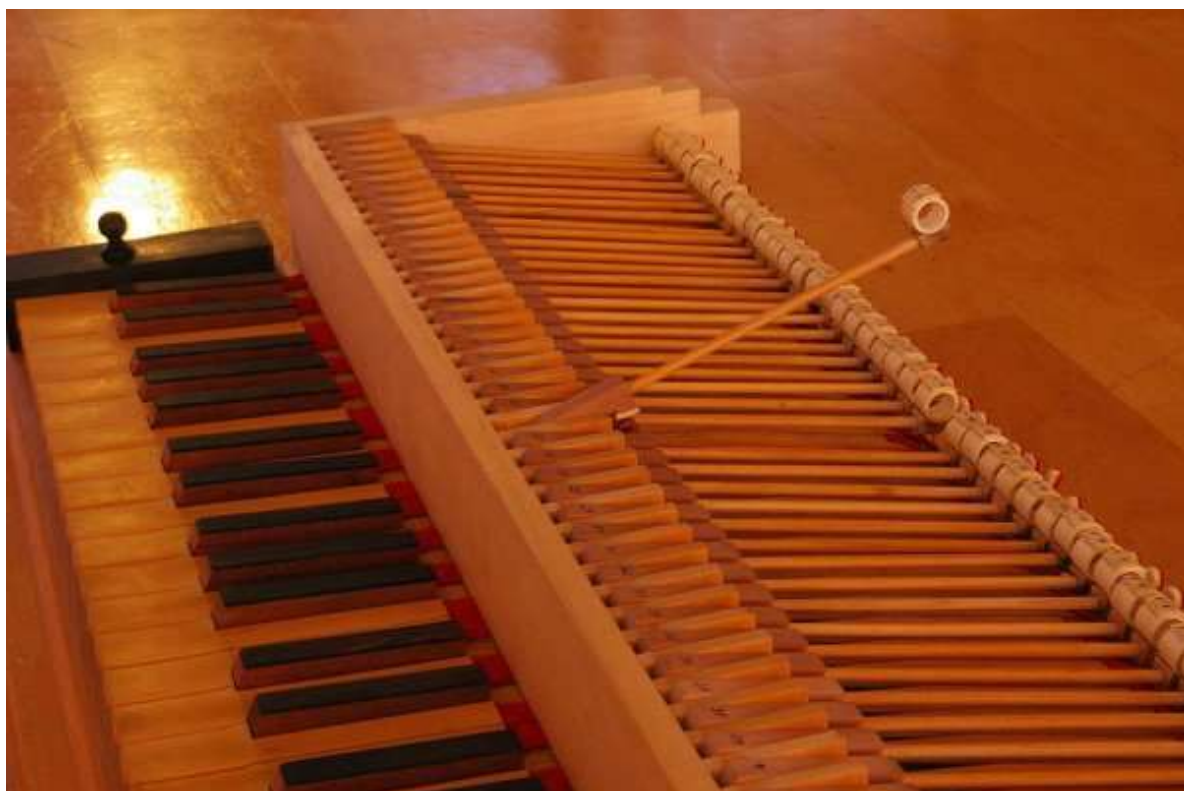
Illus.6 Hammer action of the 2000 copy by Kerstin Schwarz of the 1726 Cristofori piano (reproduced with kind permission from Kerstin Schwarz)
