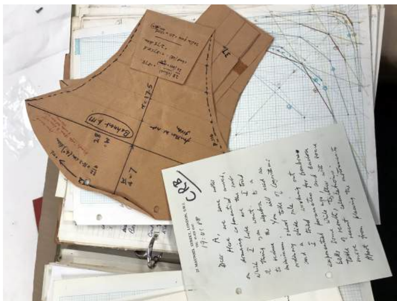
Illus.4 Templates for trombone bells (photo: Alice Little)
