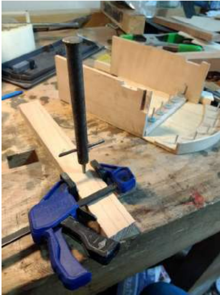
Illus.22 Using a balance pin tool, with a clamp to avoid splitting
