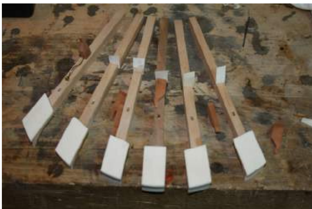
Illus.26b Key tops and escapement hinges added to keys
