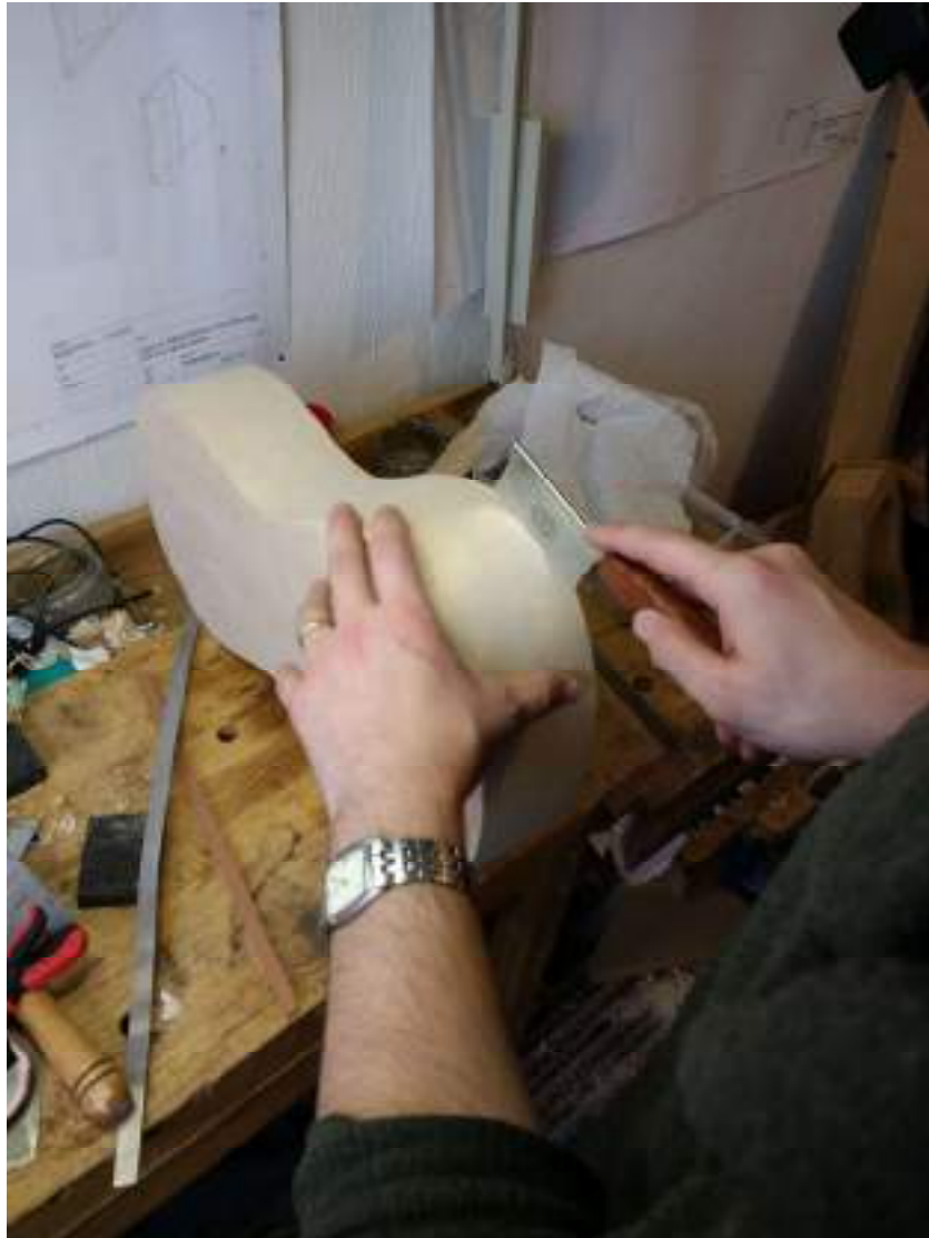
Illus.7 Cutting the opening for the mechanism with veneer saw
