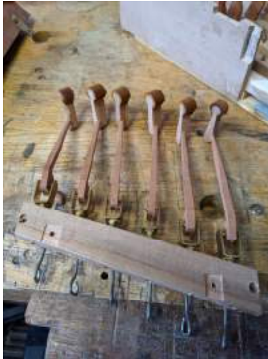
Illus.27 Hammer arm rail, with adjustment screws for the escapement
