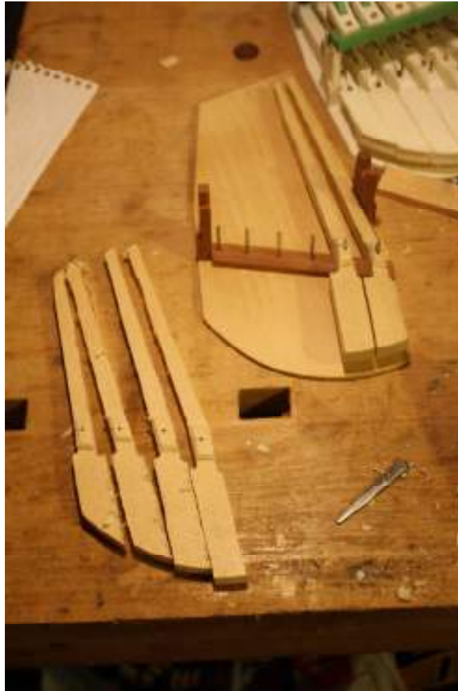
Illus.10 Keys cut out, with holes for the balance pins
