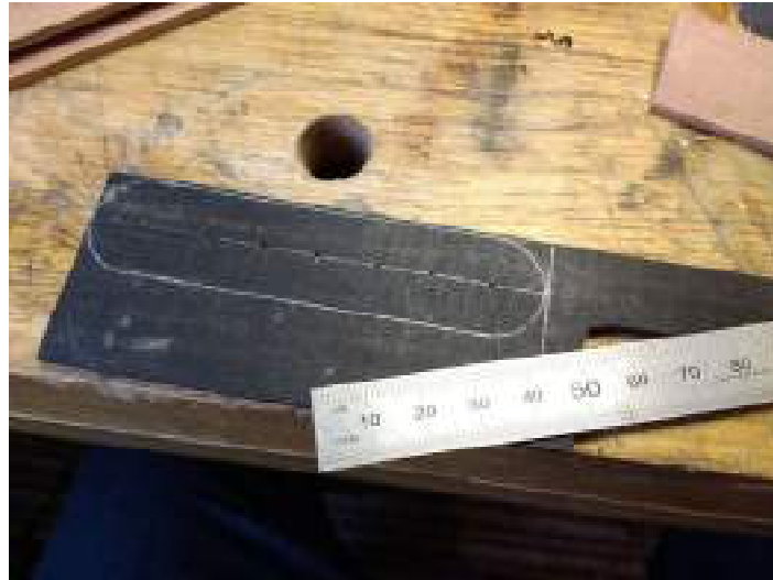
Illus.11a/ b The soundboard was prepared, and the hammer hole was roughly cut out, reinforcement made from ebony
