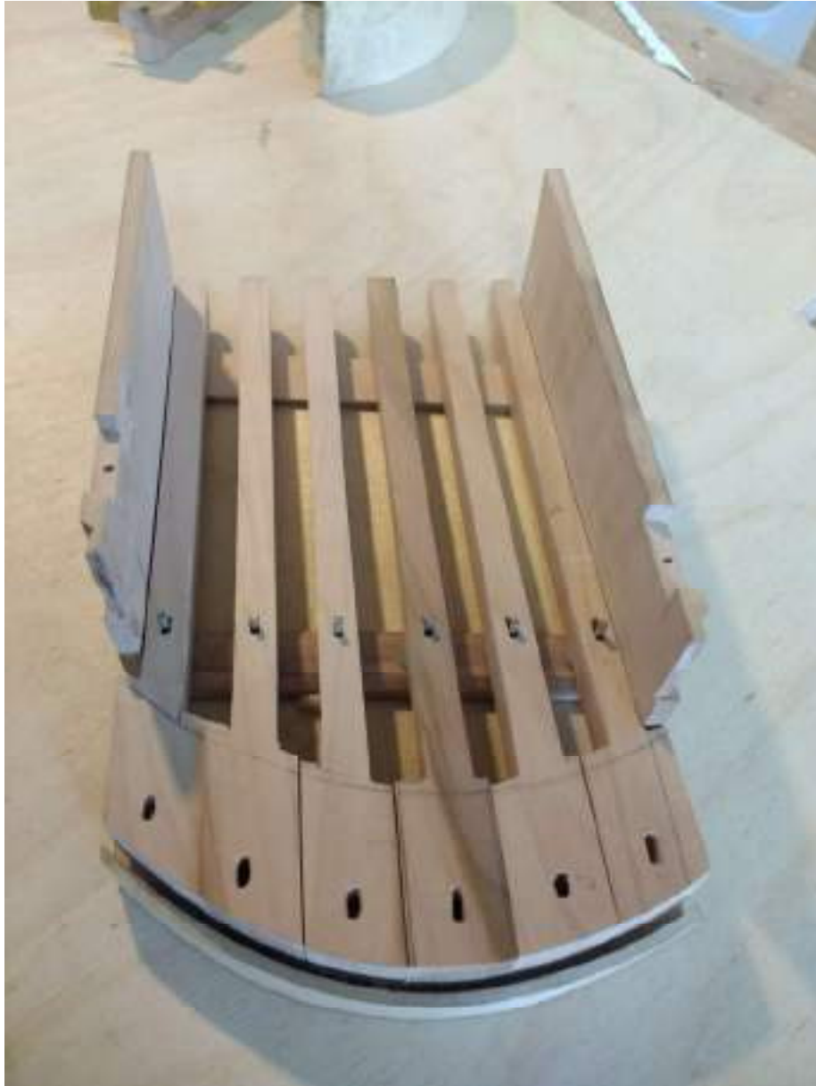
Illus.24 Keys fully shaped to fit the mechanism
